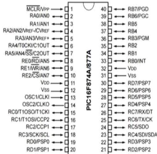
Fig. 2. Pin configuration of the PIC 16F877A microcontroller
