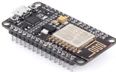
It is a development kit which has vast applications. In agriculture monitoring and data acquisition system the Node MCU is used for processing the data.
