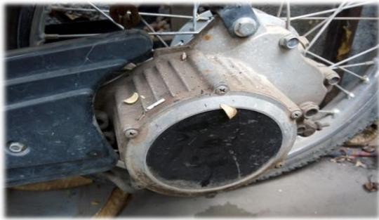
**Fig-6:** Motor Coupled with rear wheel
