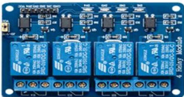
FIGURE7 - FOUR-CHANNEL RELAY BOARD
