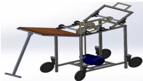
**Fig -2:** CAD model of Multipurpose Machine.
