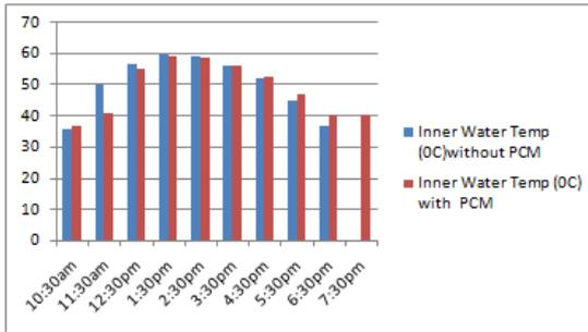
Graph No 1: Comparison of water temp with and without PCM
