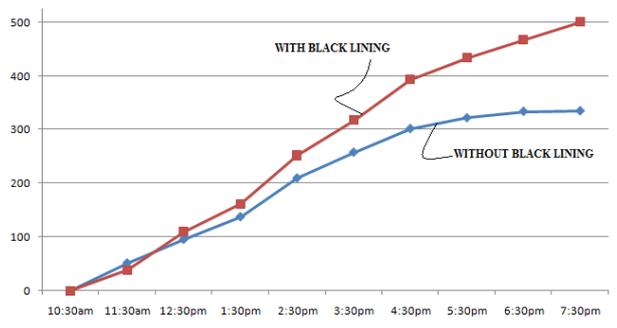
Graph No 5: Comparison of Single slope single basin solar still with and without black coating
