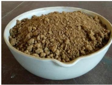
**Fig -1:** Soil used for the preparation of brick
