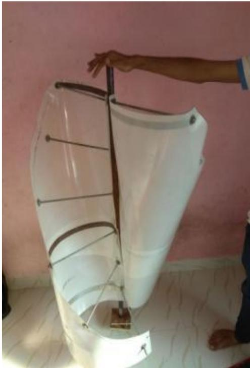
**Fig -4:** Modified Savonius Turbine
