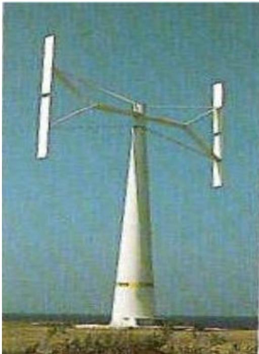
**Fig -2:** Variable Geometry Vertical Axis Wind Turbine
