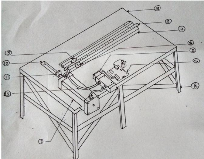
Fig. 1- Schematic Layout of Pneumatic Operated Stirrups Making Machine
