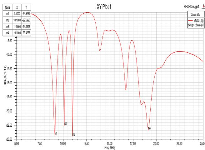
Fig 6: Return loss after last iteration
