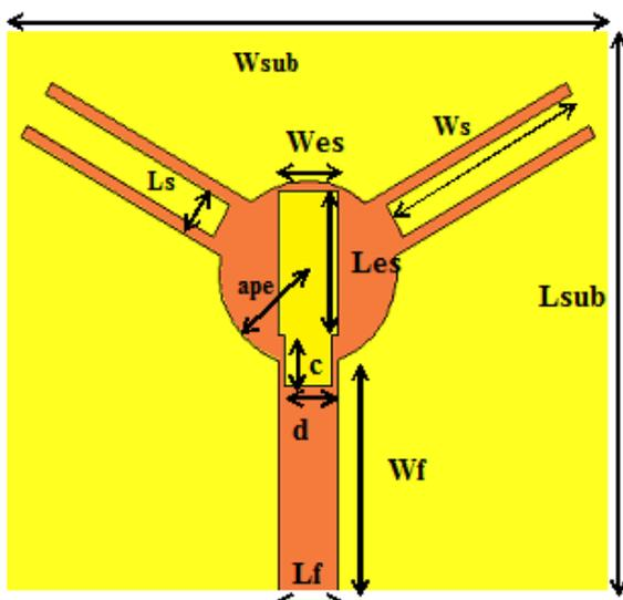
Fig -1 proposed design model - view at front
