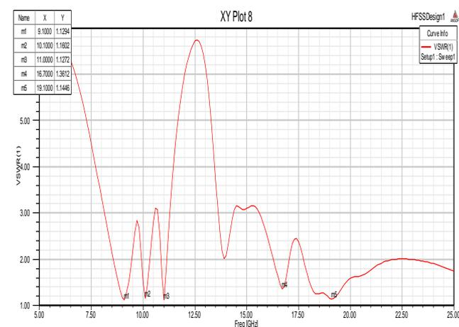
Fig 7: VSWR plot after last iteration
