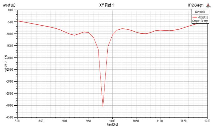
**Fig 4:** Return loss after first iteration
