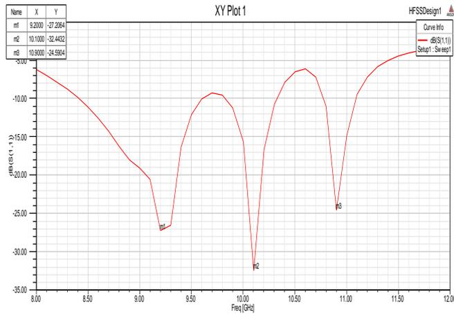
Fig 5: Return loss after second iteration
