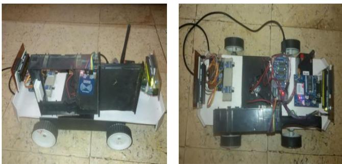
**Fig -4:** Prototype model of driverless metro train
