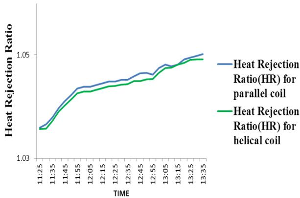
Chart -9: Heat rejection ratio For parallel Vs Helical coil condenser
