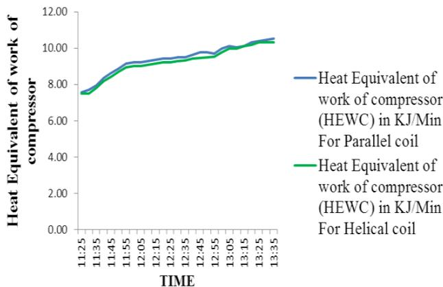
Chart -4: Equivalent work For parallel Vs Helical coil condenser
