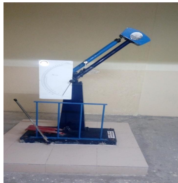
Fig. 3 Experimental set up of charpy impact testing.
