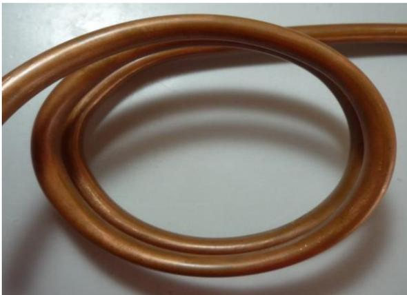
Figure 8: Result with water filled tube on rubber mandrel
