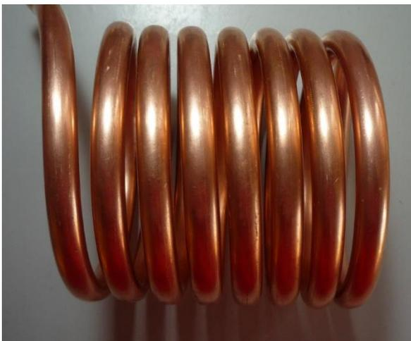
Figure 9: Result with salt filled tube on rubber mandrel
