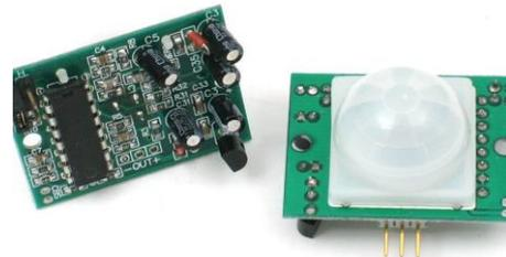
Figure 3. PIR motion Sensor
