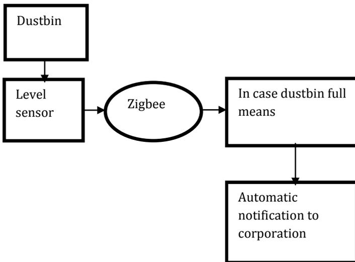
Figure 3: This shows how the dustbin works with the help of sensors
