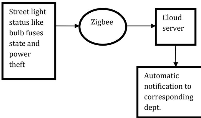
Figure 2 : This shows how the notification is generated over the zigbee technology.
