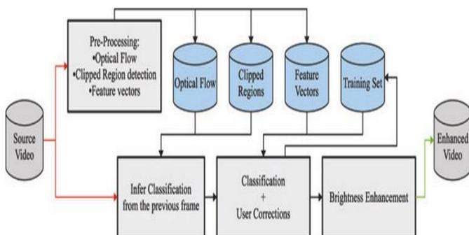
Fig - 2: System architecture of source LDR to enhanced HDR.
