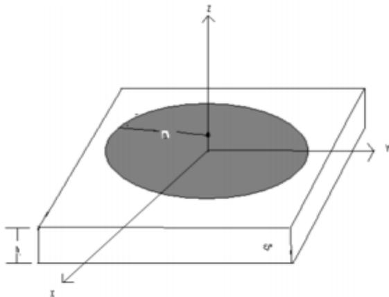
Fig1 Geometry of circular patch antenna
