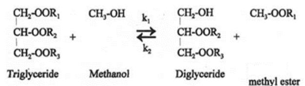
Fig.1. Reaction of triglyceride reacting with methanol
