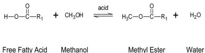
Fig.2.Reaction of Fatty acids reacting and methanol
