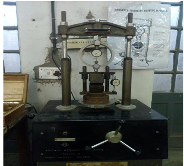
Fig.2: Marshall Apparatus for Sample testing.
