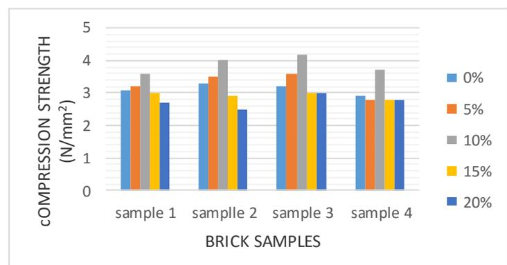
**Chart 1** Compressive Strength of Fly Ash Bricks
