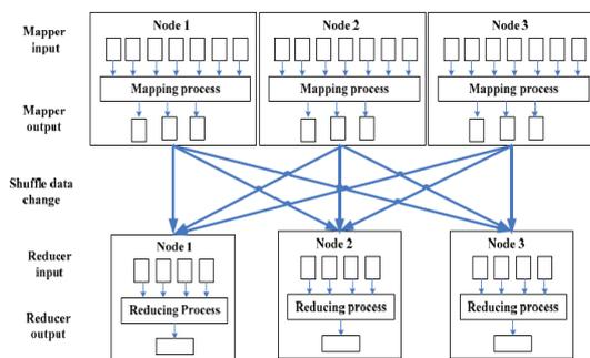
Fig. 5 the implement system of the Map/Reduce stream
