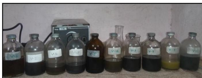
Fig -3: Samples of viscosity test
