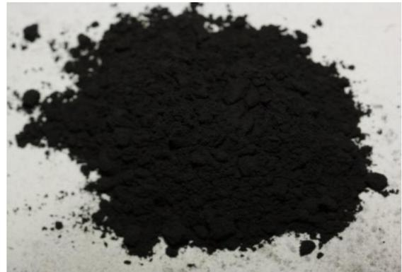
**Fig -1:** Copper oxide (CuO) in form of nano powder
