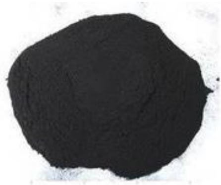
**Fig -2:** Molybdenum disulphide (MoS<sub>2</sub>) in form of nano powder
