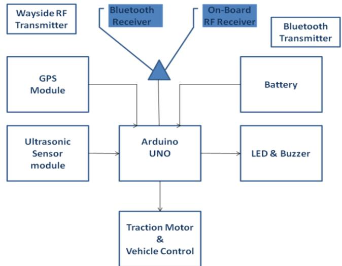
Fig -3 : Functional Block Diagram of Automated Speed Control of Auto motives
