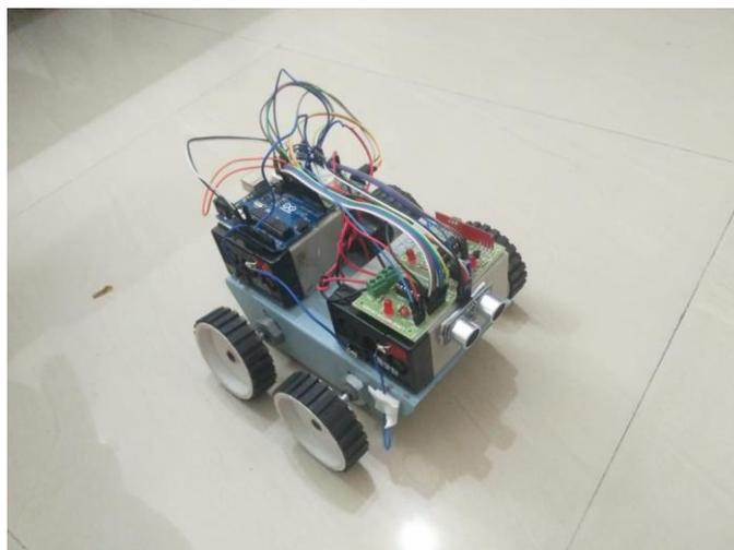
Fig -2 : Real time Prototype of automatic speed controlled car
