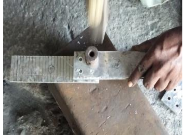
Fig -4: Preparation of riveted joints
