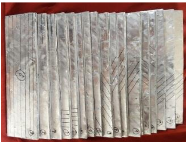
Fig -3: Aluminum -Glass fiber composite 18 Sample of Specimens
