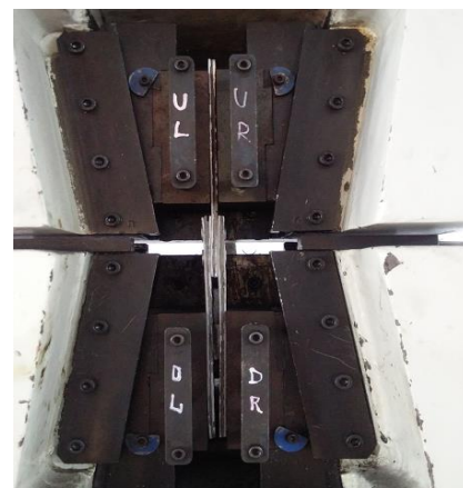
Fig -5: UTM machine Sample loaded condition for tensile testing.
