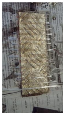
Fig -1: 45° Fibre Orientation Fig -2: 0° Fibre Orientation
