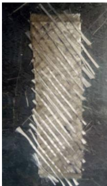
Fig -1: 45° Fibre Orientation Fig -2: 0° Fibre Orientation
