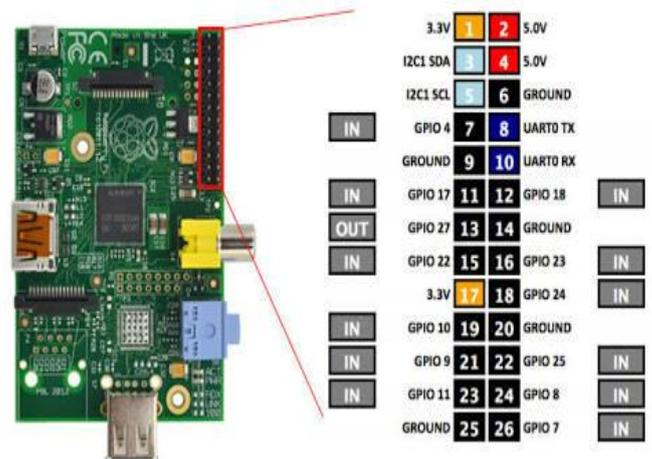
Fig.2 Pin diagram of raspberry pi
