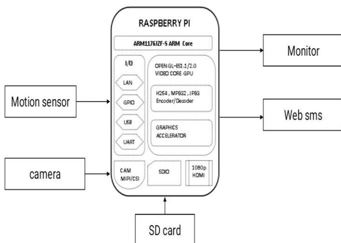
Fig 1. Block diagram of CCTV Camera
