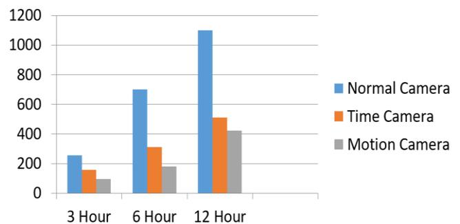
Fig 4. Comparison of memory storage of various camera
