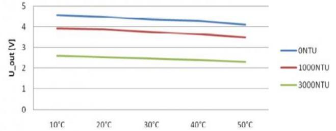
Figure 3. Voltage-Temperature characteristic
