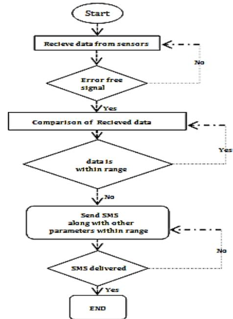
Figure 4. Flow chart of alert system
