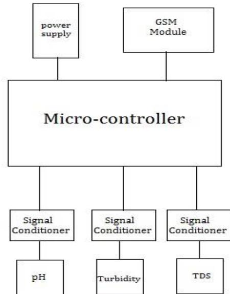
Figure 1. Design of System
