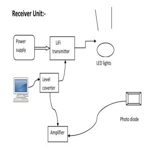
The required data sent by the user is received by the server by means of photodiode and level converter. The server reads the data required by the user and then transmits it by means of lifi transmitter to the user by using LED lights.
