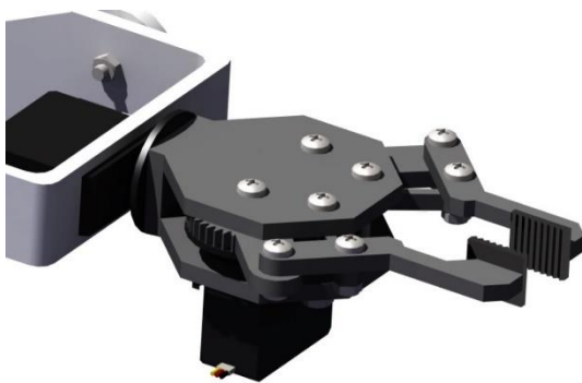
Fig – 6: End effector powered by servo in the robotic arm
