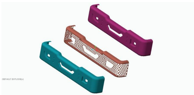
Fig 3: Assembly of bumper with honey comb
