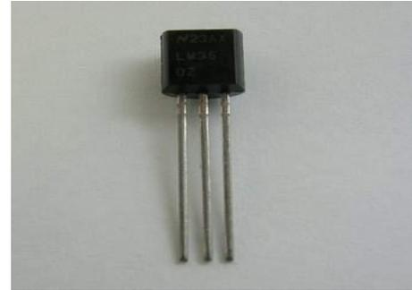
Fig.5 Temperature Sensor
