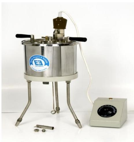
Fig-2 Say bolt Viscometer.
