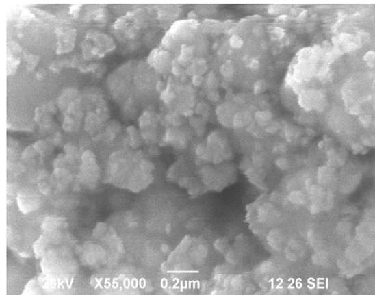
**Fig-1 SEM image of ZnO nanoparticle at 0.2micrometers**
