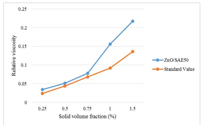
Fig-4 Volume fraction vs Relative Viscosity
