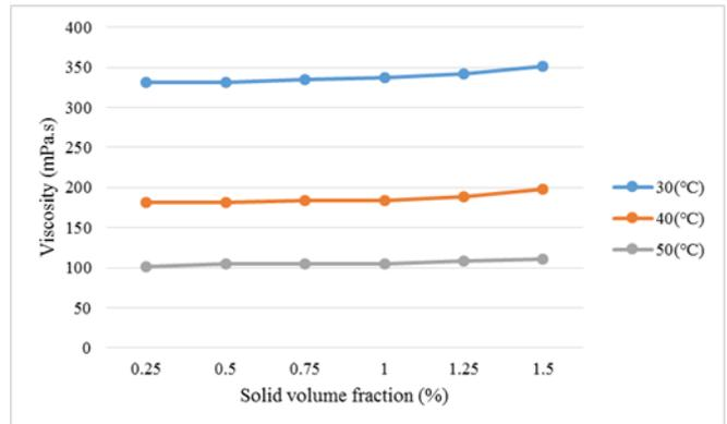
Fig-3 Volume fraction vs Viscosity
