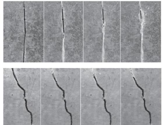
Surface images of specimens with crack and after repair
