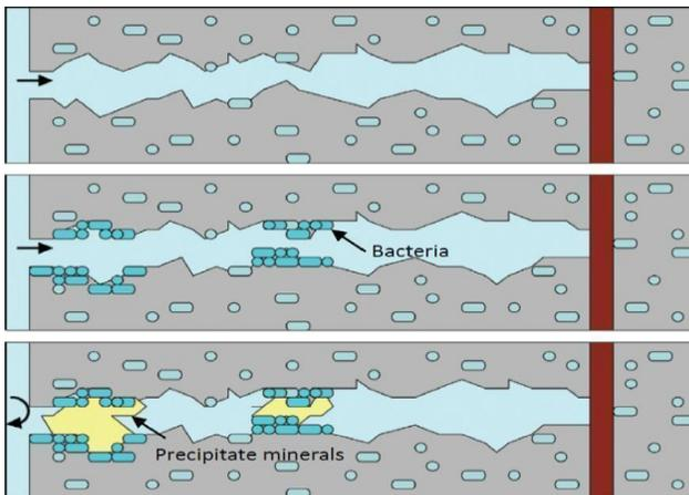
**Schematic scenario of crack-healing by concrete-immobilized bacteria**
