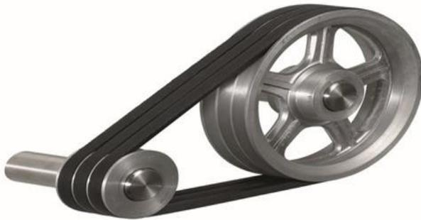
Fig-2: Belt & Pulley Drive
