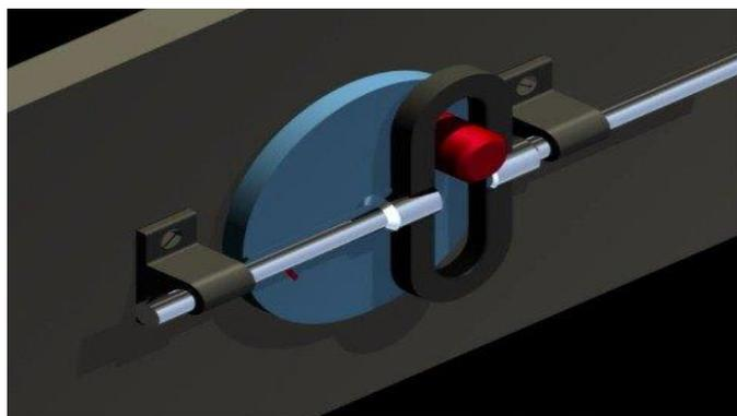
Fig 4: Scotch Yoke Mechanism
