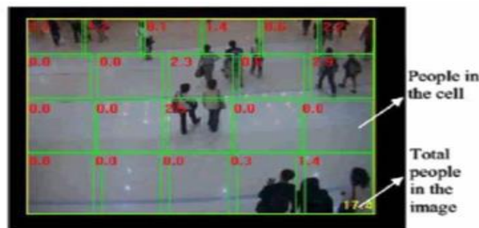
Fig -4: Multi-resolution density cells indicating the estimated numbers of people in individual cell and entire region.
