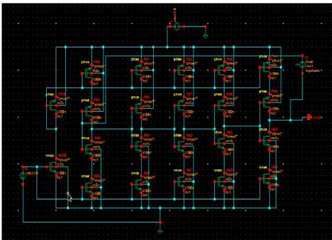
Fig 3.1 Schematic View of CSVCO
