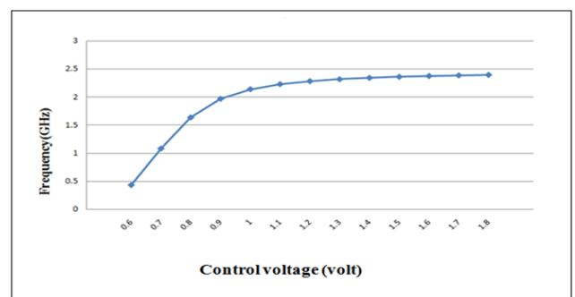
Fig 3.3 Graphical Representation of Output Frequency VS Control Voltage
