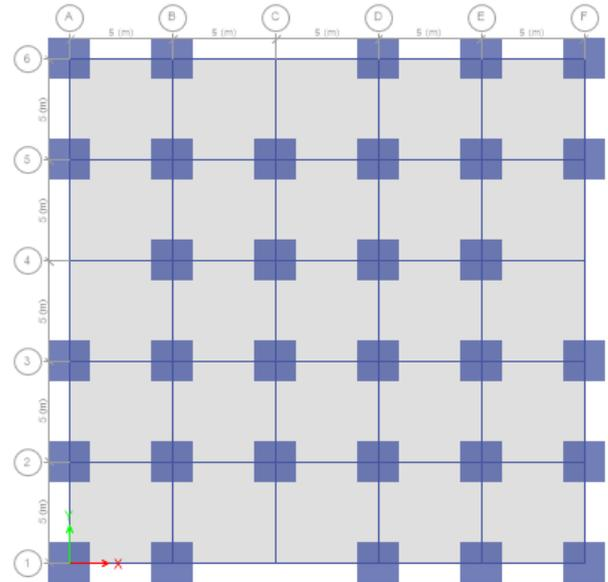
**Fig-2:** Plan view with floating column at exterior side of frame
