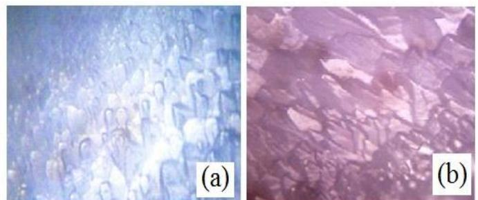
Fig – 9: Etching pattern of as grown A4MBS
