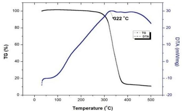
Fig – 8: TG-DTA curve of A4MBS
