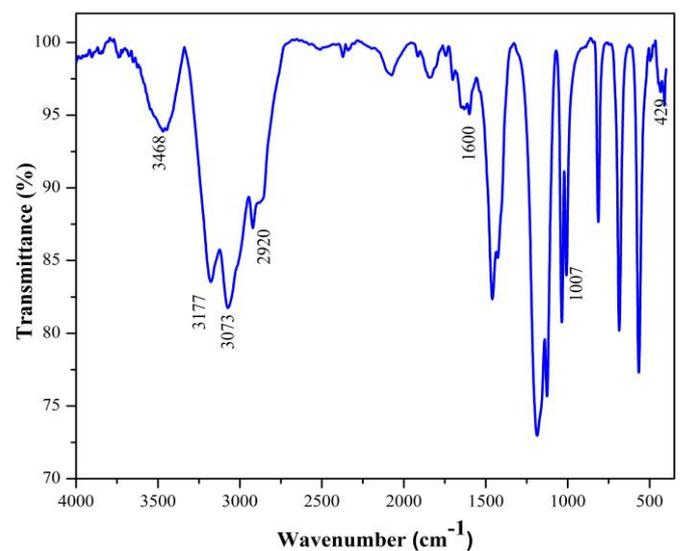
Fig.4: FT-IR spectrum of A4MBS
