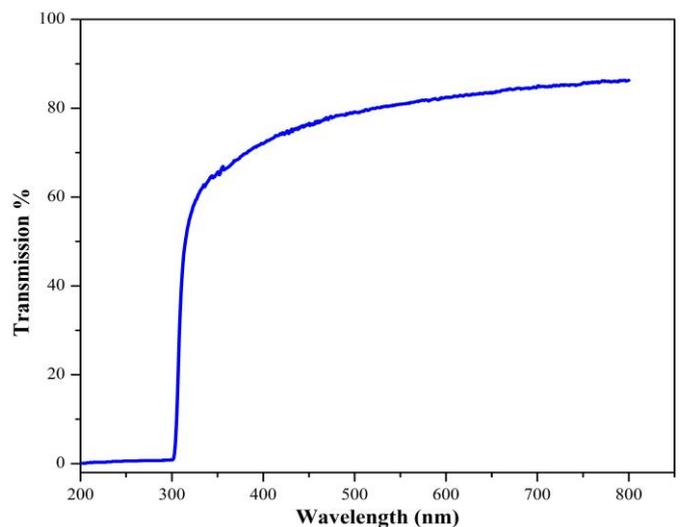
Fig - 7: UV transmission spectrum of A4MBS
