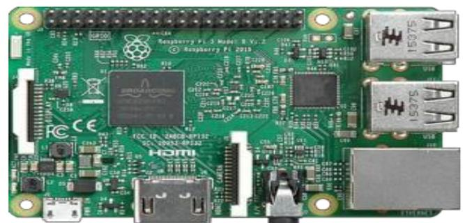
Fig-1.1 RaspberryPi3ModelB board
