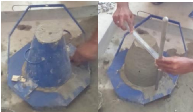
Fig 2: Slump Cone Test
