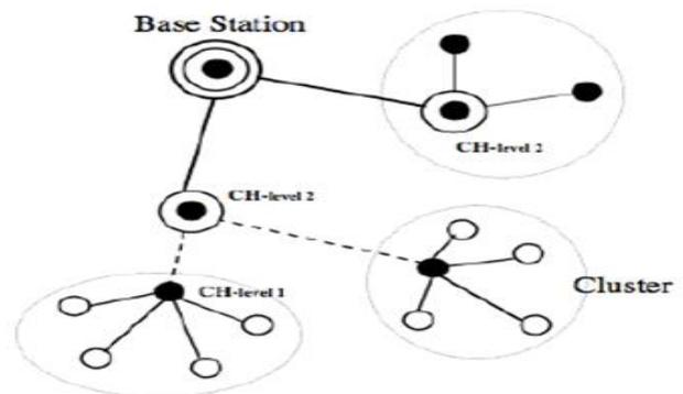
Fig -3: Cluster Based Hierarchical Model
