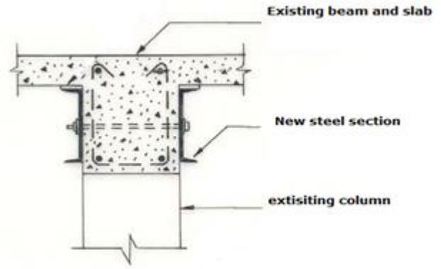
Fig.4 Adding steel section on existing concrete beam
