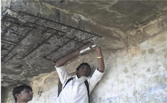
Fig.8 Rebound hammer test carried out on beam of Bal vihar
