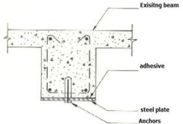
Fig.12 strengthening of the existing beam
