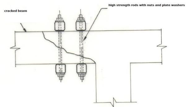
Fig. 5 Cracked beams
