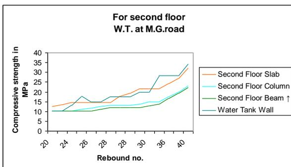
Fig. 3 Rebound hammers results for second floor of water tank
