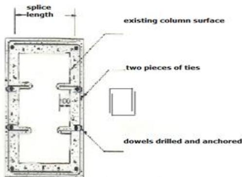
Fig.11 strengthening of the existing column
