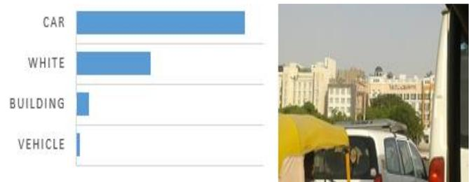
We integrated tensorflow in Android studio with our trained model. And it is deployed in raspberry pi with the help of Android Things Operating System.
