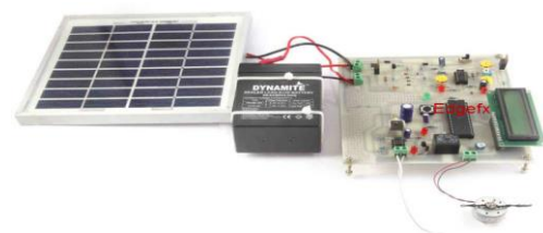
Figure 6: Solar Powered Auto Irrigation System Circuit
