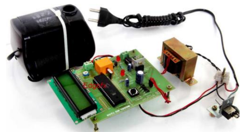
Figure 4: Automatic Irrigation System Kit
