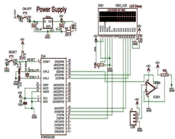
Fig 2: Receiver section
