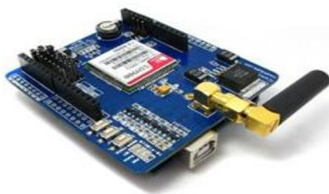
**Fig-3:** GSM Module
