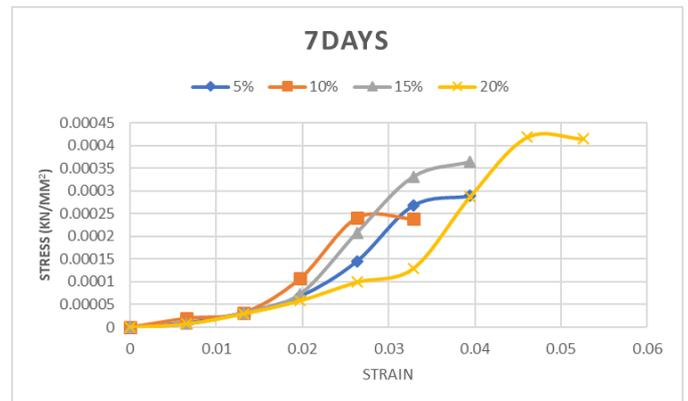
Chart -5: Compressive stress strain curve for 7 days curing
