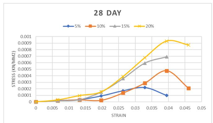
Chart -6: Compressive stress strain curve for 28 days curing
