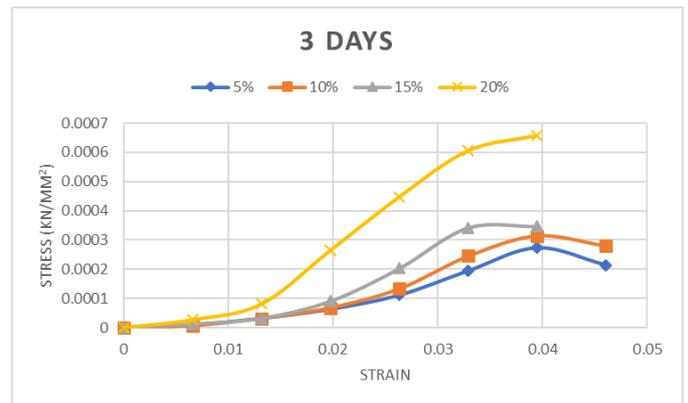
Chart -4: Compressive stress strain curve for 3 days curing
