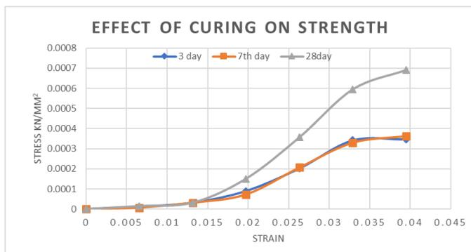
**Chart -7:** Effect of curing period on the sample containing 15% cement
