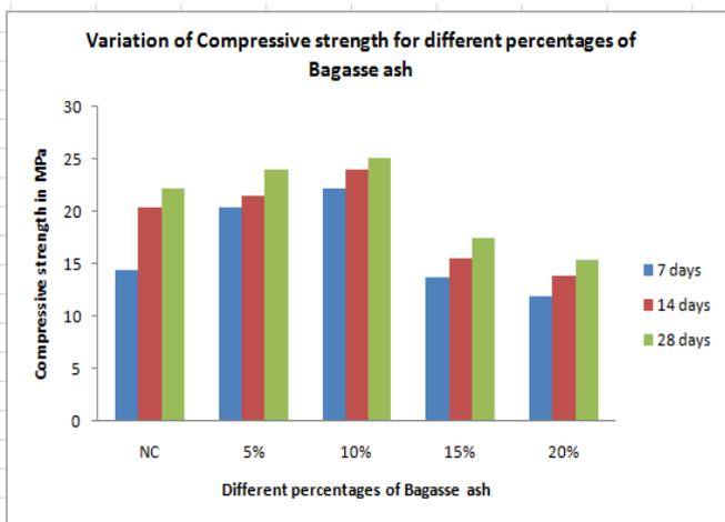
The above graph indicates that the compressive strength of 7 days, 14 days, 28 days with 0%, 5%, 10%, 15% and 20% percentage of bagasse ash replaced in cement and quarry dust replaced with fine aggregate in the concrete mixes. The normal concrete give a compressive strength compared to different days of curing. Strength of concrete increases with increase in percentage of replacement of Bagasse ash up to 10% and thereafter decreases with remaining percentages of Bagasse ash.
