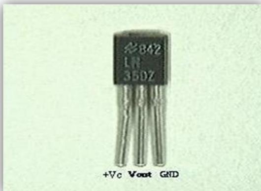
**FIGURE 1: LM35 TEMPERATURE SENSOR**
