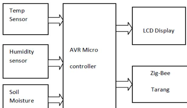
**FIGURE5: BLOCK DIAGRAM OF TRANSMITTER SIDE**
