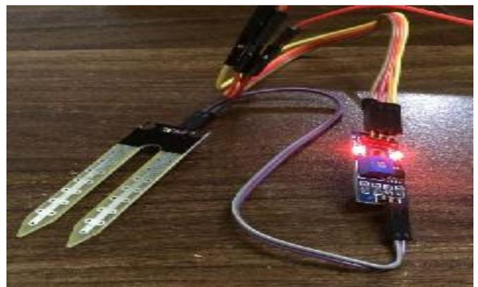
**FIGURE 3: SOIL MOISTURE SENSOR YL38**
