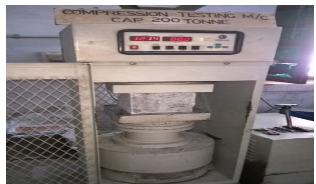
Figure-2: Specimen testing in Compression Testing Machine
